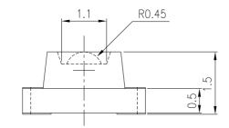
For reflow soldering (propose)
