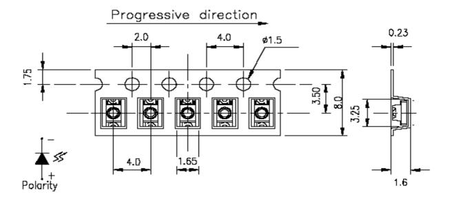
**Note:** The tolerances unless mentioned are  $\pm 0.1$ , Unit = mm.
